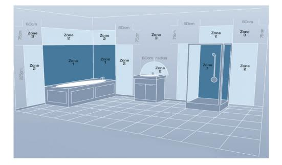
Zone1 – Can not be installed the electric radiators with thermostat or with on/off switch!
